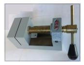
This screw type drill vise is also Machine vise. This vise is made of C.I. And working capacity of vise is 76.20mm length, width is 76.2mm and height is 45mm.
